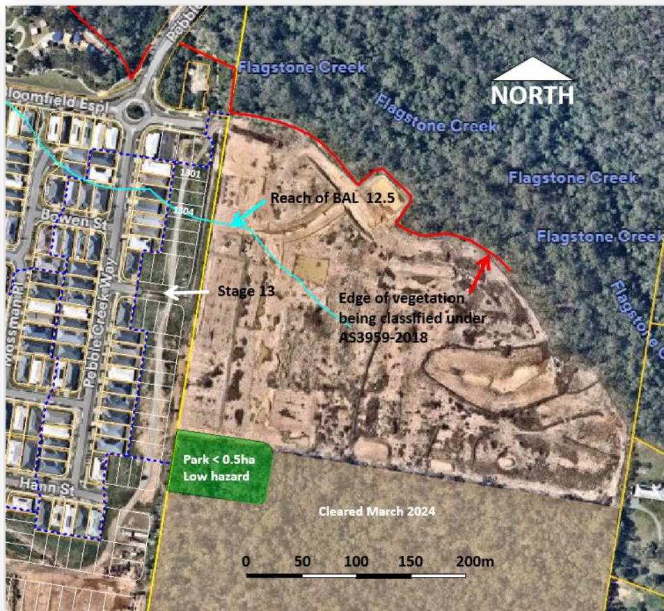
Figure 1. The effect of recent clearing on construction requirements for Stage 13
